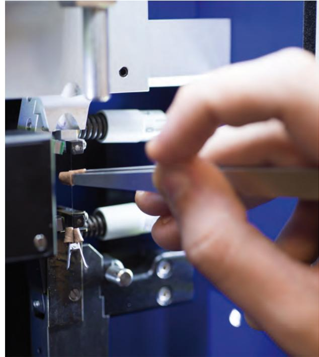
Figure 1: Single filament test on carbon fibres
