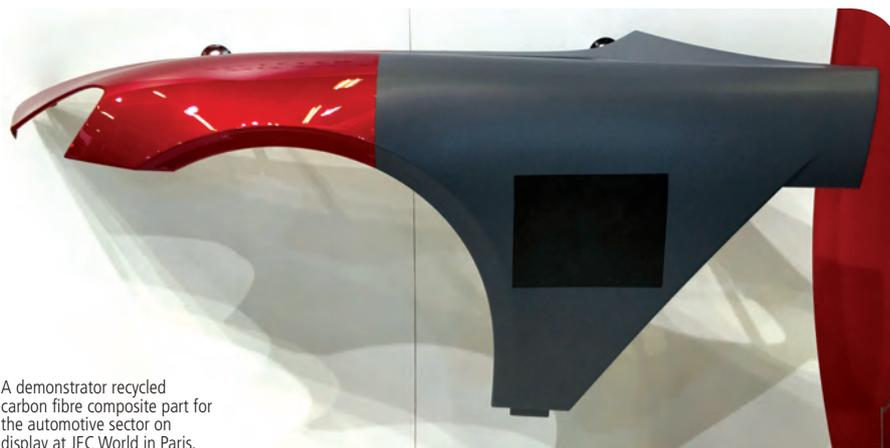
A demonstrator recycled carbon fibre composite part for the automotive sector on display at JEC World in Paris.
