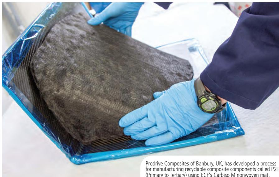
Prodrive Composites of Banbury, UK, has developed a process for manufacturing recyclable composite components called P2T (Primary to Tertiary) using ECF's Carbisio M nonwoven mat.
