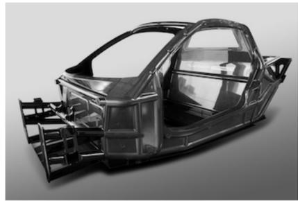
Recycled materials were used in Gordon Murray Design's CFRP-intensive iStream Carbon chassis
