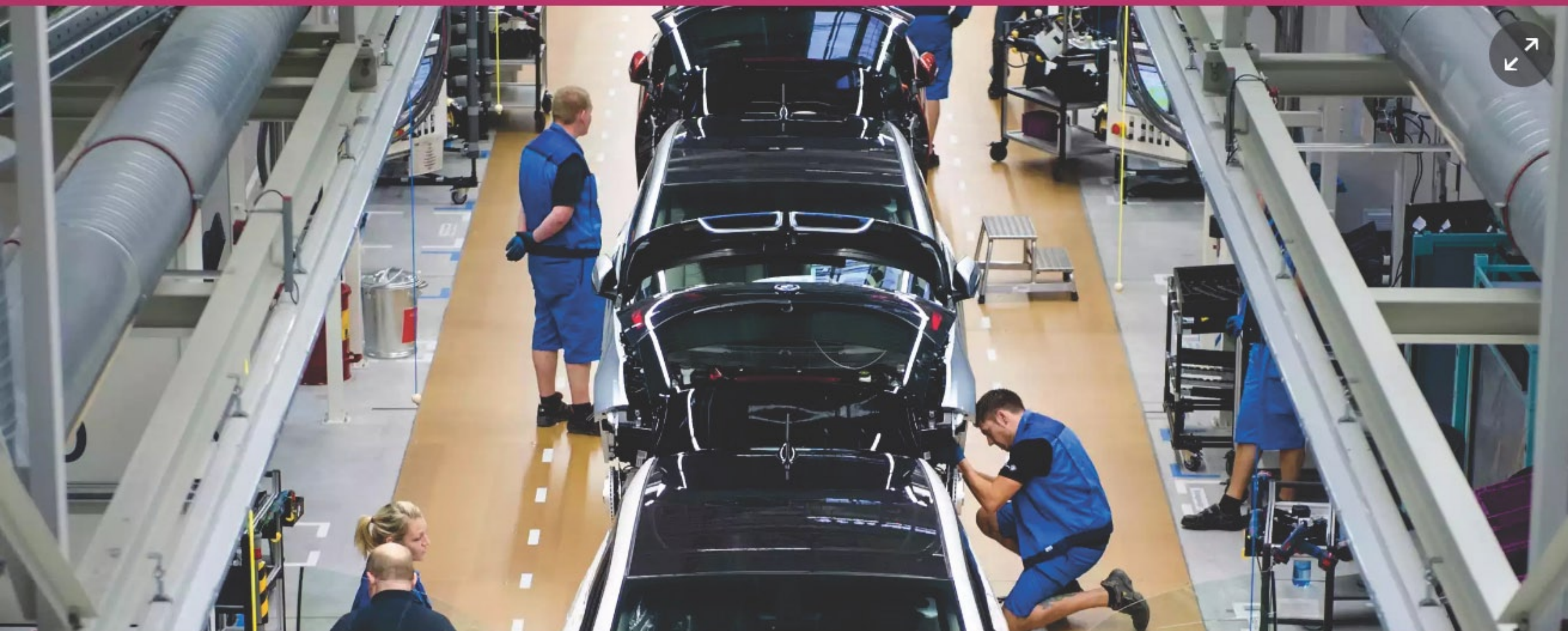
Workers in Leipzig assemble a BMW i3 electric model, the first mass-produced car with a carbon fibre passenger cell. Photograph: Jens Schlueter/Getty
