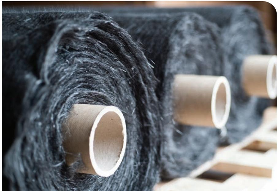
can be liberated from an epoxy laminate by boiling it in concentrated nitric acid for several hours (ISO 14127). It has also been proven that a supercritical acetone/water mix (320 °C, 170 bar) also dissolves the resin. Neither method has been scaled up to tonnage quantities and there are still significant challenges to be addressed before this technology becomes commercially viable.
