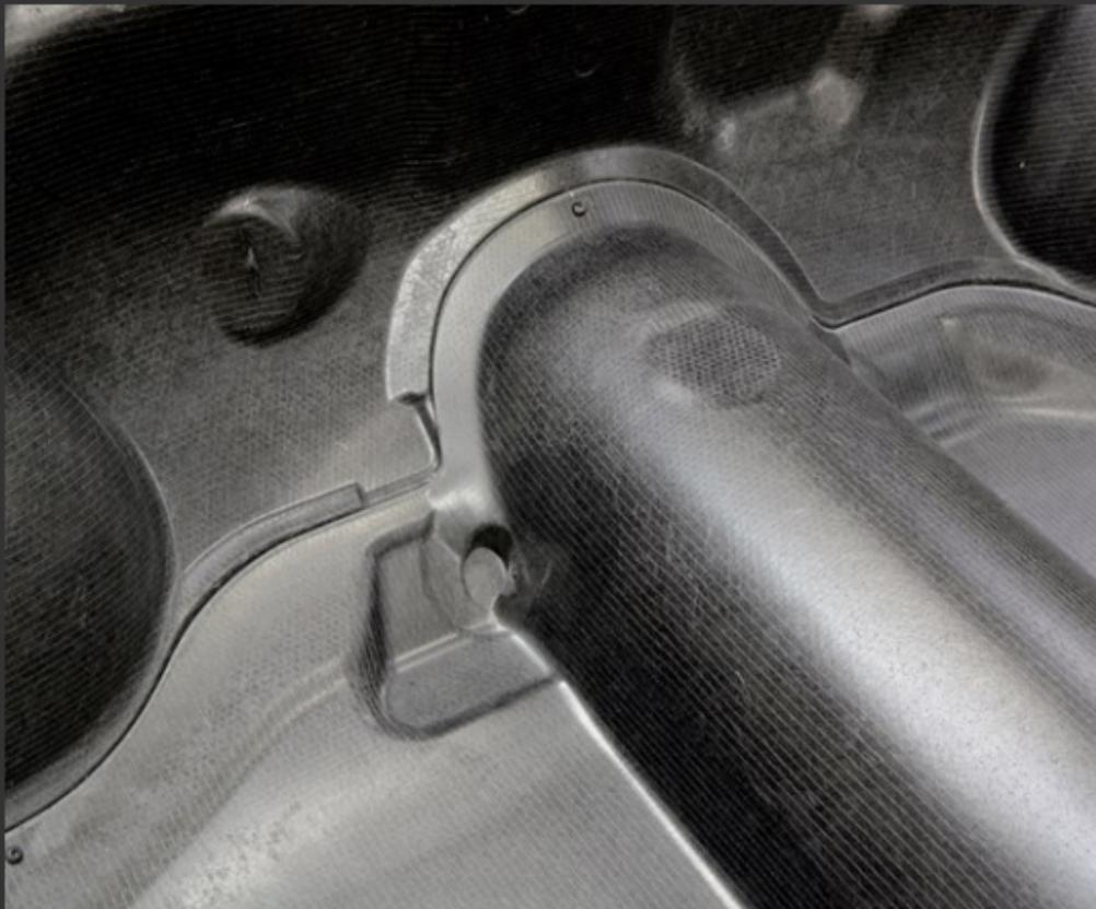
A section of BLS's Xenos chassis. ELG's recycled carbon fiber mat is beneath the surface layer of NCF that can be clearly seen. Only a small number of mechanical fasteners are used to hold the five separate sections together, while adhesive is injected into the tongue and groove joints.
